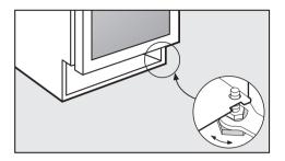
Align the appliance to the height of the niche by altering the adjustable feet using the spanner supplied.
